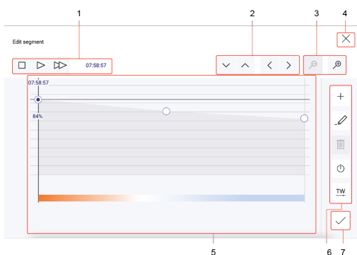
Figure 7: "Edit segment" view > segment from a curve for TW luminaires > intensity can be edited
