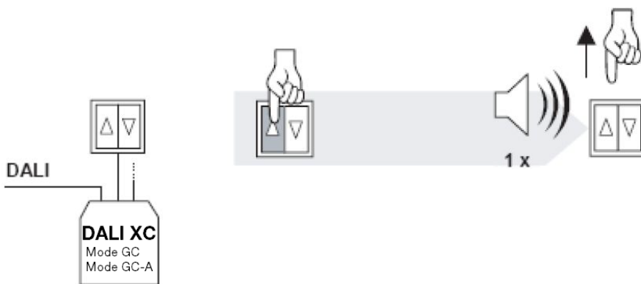
Figure 5: Assigning a luminaire to a group
