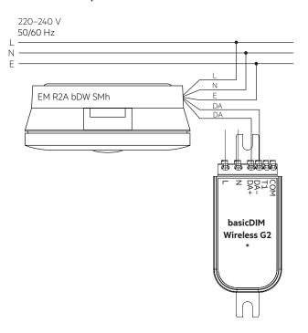
Note: Battery must be connected before mains connection.
