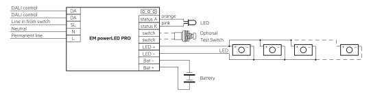
Take care that the LED is connected with the right polarity. LED that are connected to the EM powerLED PRO EZ-3 devices should have a reverse polarity protection device such as a schottky diodes fitted, otherwise irreversible damage could occur if the LED is connected in reverse polarity. Any protection device must be capaple of handling in excess of 700 mA.
