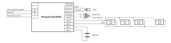
Take care that the LED is connected with the right polarity. LED that are connected to the EM powerLED devices should have a reverse polarity protection device such as a schottky diodes fitted, otherwise irreversible damage could occur if the LED is connected in reverse polarity. Any protection device must be capaple of handling in excess of 700 mA.
