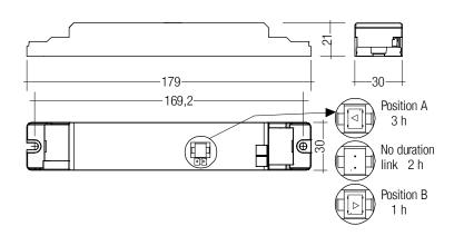
Note: LED driver supplied with duration link in 3 hours position. Duration link must be set before battery and mains connection.
