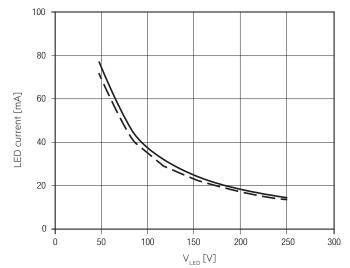
EM converterLED ST 205 MH/LiFePO4 250V Article number: 89800636 NiMH battery, 6.0 V battery voltage 820 – 880 mA battery discharge current (tolerance) LiFePO<sub>4</sub> battery, 3.2 V battery voltage 1,695 – 1,825 mA battery discharge current (tolerance)
