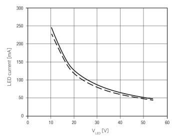
EM converterLED PRO 204 NiCd/NiMH 50V Article number: 89800651 4.8 V battery voltage 800 – 860 mA battery discharge current (tolerance)
