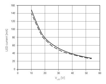
EM converterLED PRO 203 MH/LiFePO4 50V Article number: 89800628 NiMH battery, 3.6 V battery voltage 890 – 960 mA battery discharge current (tolerance)
