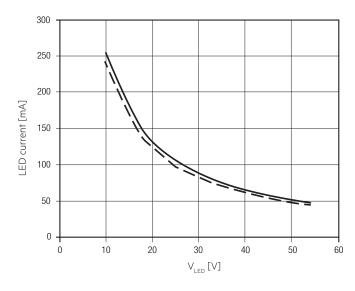
EM converterLED PRO 204 MH/LiFePO4 50V Article number: 89800629 NiMH battery, 4.8 V battery voltage 785 – 845 mA battery discharge current (tolerance)
