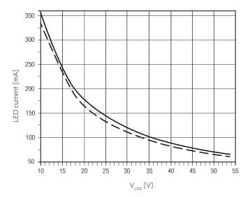
EM converterLED BASIC 203 MH/LiFePO4 50V Article number: 89800576 LiFePO<sub>4</sub> battery, 3.2 V battery voltage 1,150 – 1,250 mA battery discharge current (tolerance)
