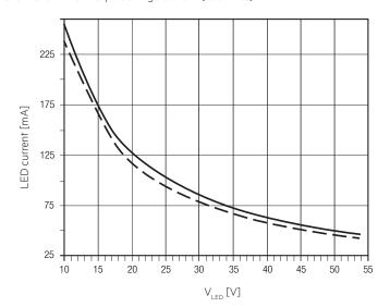
EM converterLED BASIC 204 MH/LiFePO4 50V Article number: 89800577 NiMH battery, 4.8 V battery voltage 825 – 885 mA battery discharge current (tolerance)
