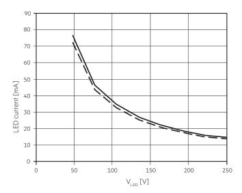
EM converterLED BASIC 205 MH/LiFePO4 250V Article number: 89800582 NiMH batteries, 6,0 V battery voltage 860 – 920 mA battery discharge current (tolerance) LiFePO<sub>4</sub> batteries, 3,2 V battery voltage 1770 – 1900 mA battery discharge current (tolerance)
